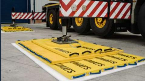
Engaged patented interlock
