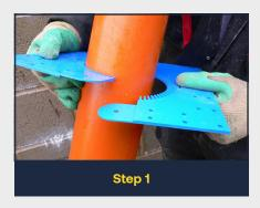
1 - Attach the Instant Pipe Shutter to the pipe
