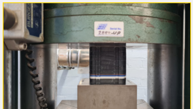
Photo of 80mm shim stack under 143.8kN load
